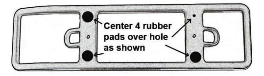
Install 4 self-adhesive rubber pads on the inside of each side panel
